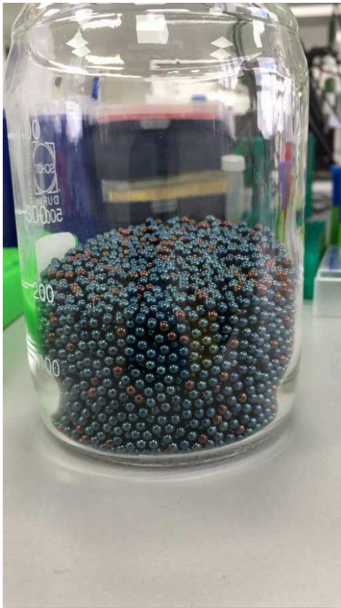
Figure 1: Depending on baking time, carbon steel beads will change colour, this is normal.
