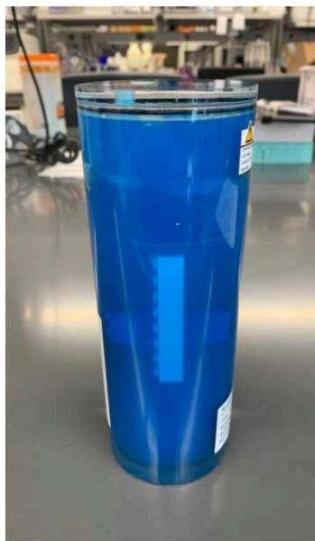
Geometric phantom (radius = 35 mm and height = 190 mm)
