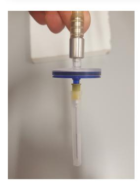
Attach the vials by piercing the stoppers with the attached needles.
