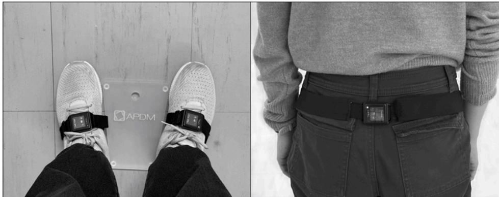
**Figure 2:** The wearable sensors to measure gait speed are attached to the right and left foot (each centered on the top of the foot) (left panel) and in the midline just below the waist at the level of the second sacral spinous process (S2) (right panel). S2 is at the level of the posterior superior iliac spine. Ensure the port is facing downwards. The starting position of the feet is standardized by positioning them adjacent to the docking system.
