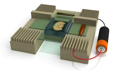
The bottom glass contains the tissue and is placed on top of the EEL holder. This is the capture slide and is connected to the positive pole of the power source (here depected as a battery) with the red wire and the coper tape. Two PDMS spacer separate the sample with the top electrode, which is connected to the negative pole with the black wire and coper tape. Pipett the electrophoresis buffer intbetween the glasses.
