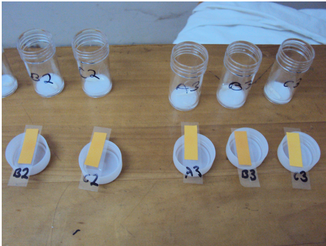
Figure 5: Labeled picrate papers that were left to dry on screw cap lids
