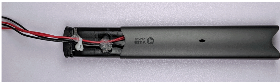
ENDS PCU inner plastic carrier sliding into the ENDS PCU outer metal case.
