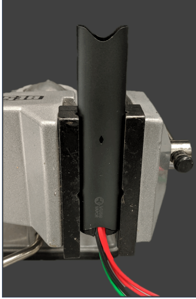
(A) ENDS test fixture held vertically using table top vise.
