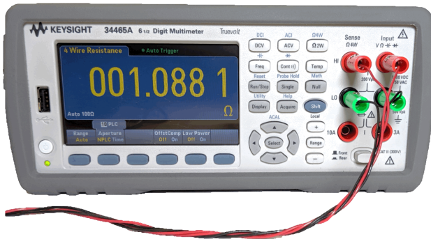
(B) ENDS test fixture leads plugged to Keysight 34465A DMM.
