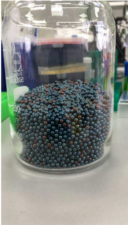
Figure 1: Depending on baking time, carbon steel beads will change colour, this is normal.
